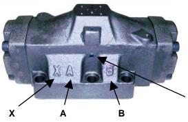
View the valve in the orientations shown. (The valve is shown without the pilot valve.)
