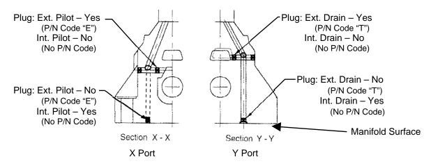
At conversion, the one plug that is removed may be used as the other required plug.
